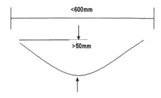
d) Carriageway – Bituminous - Change of carriageway profile greater than 50mm and extending in plan direct less than 600mm
