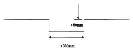
e) Carriageway - A depression (pot hole) of 50mm or greater in depth and extending in any one direction greater than 300mm may constitute a safety hazard
